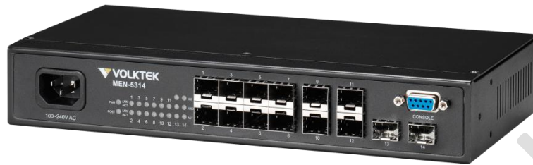
12-slot 100Base-FX SFP + 2-slot Gigabit Multi-rate SFP
