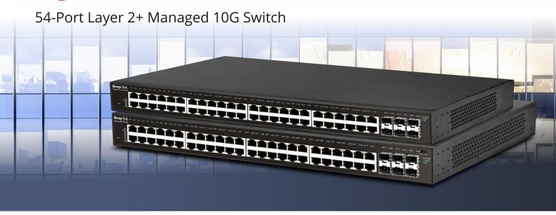
DrayTek VigorSwitch 2540x series is a Layer 2+ Managed 10 Gbps switch with 48 Gigabit Ethernet ports and 6 x SFP+ 10Gbps Fiber links. Supporting advanced Layer 3 features, DHCP Server and VLAN Routing. Moreover, it supports VLAN routing to route the inter-VLAN traffic directly, shares loads of the router, and improve overall network performance.
