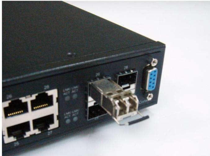
3) Insert and slide the module into the SFP slot until it clicks into place:
