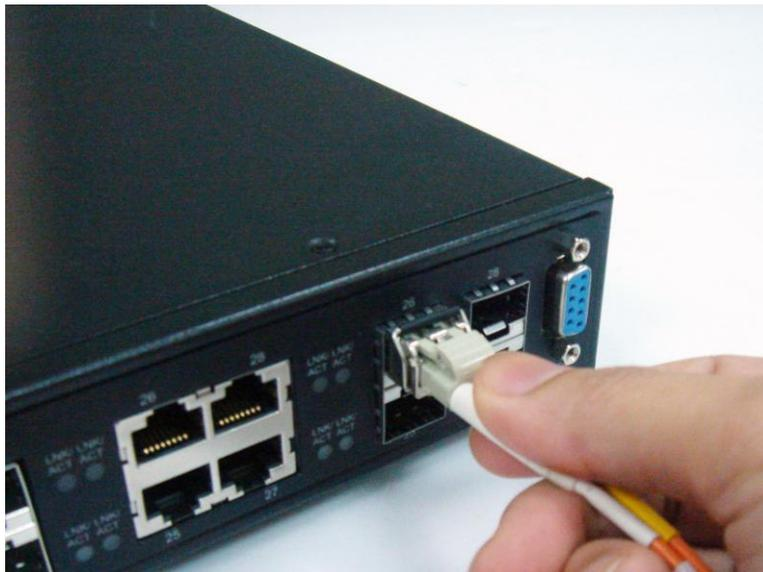
7) If you want to pull the connector out, first push down the release clip on top of the connector to release the connector from the SFP module.
