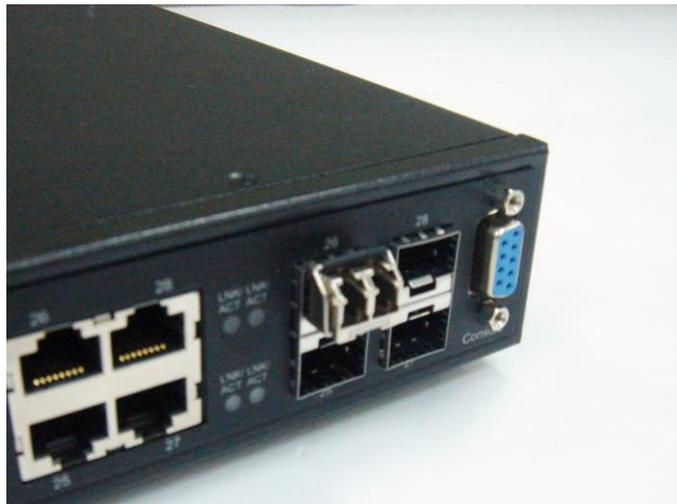
4) Remove any rubber plugs that may be present in the SFP module's mouth.
