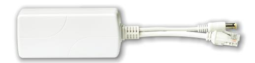
**APTEK GE122A** is a PoE (Power over Ethernet) Splitter – Used to split PoE signals into the separate network (Gigabit) and power (12VDC – 2A) signals, allowing you to connect and power the devices doesn't have PoE support by PoE switch, PoE adapter or PoE Injector.
